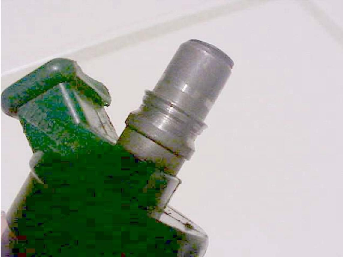
**Figure 2 Bendix injector nipple**
