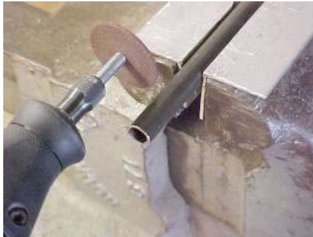
**Figure 3 Cutting spacer from brake line.**
