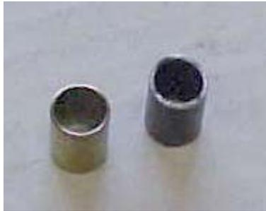
**Figure 2 Jaguar and homemade strut spacers.**
