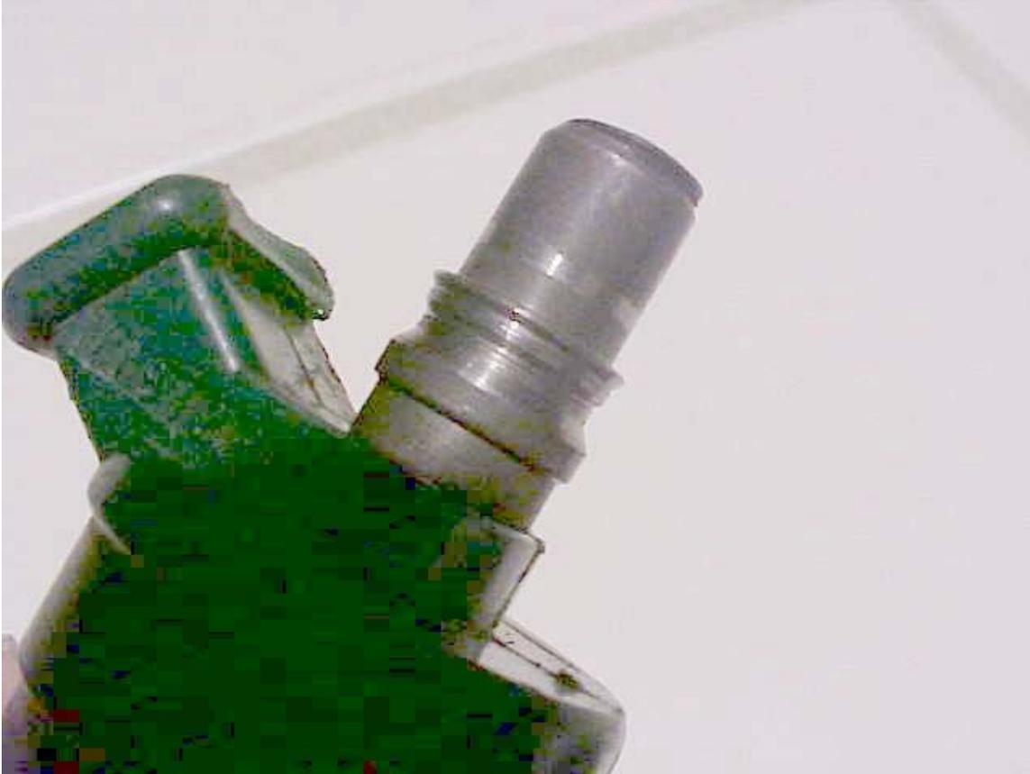
**Figure 10 Bendix injector nipple**
