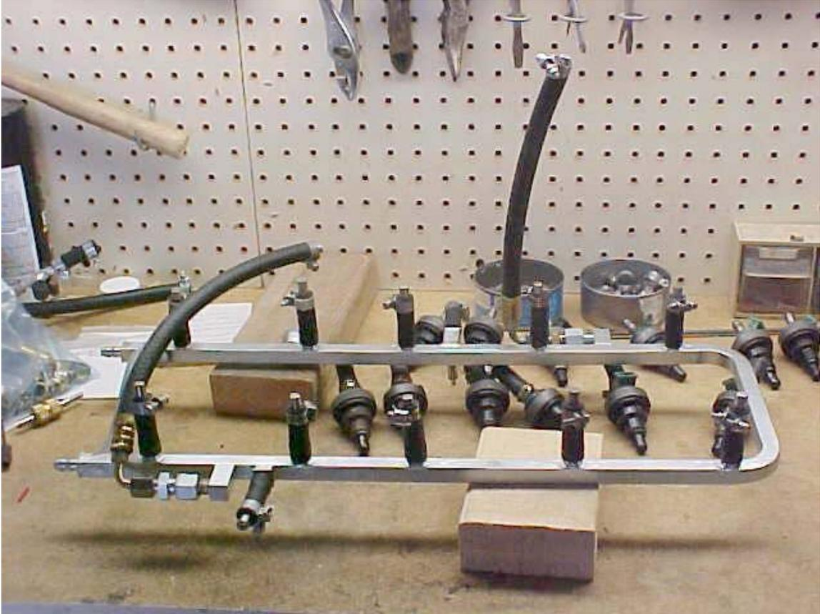
Figure 4 Testing the rail
