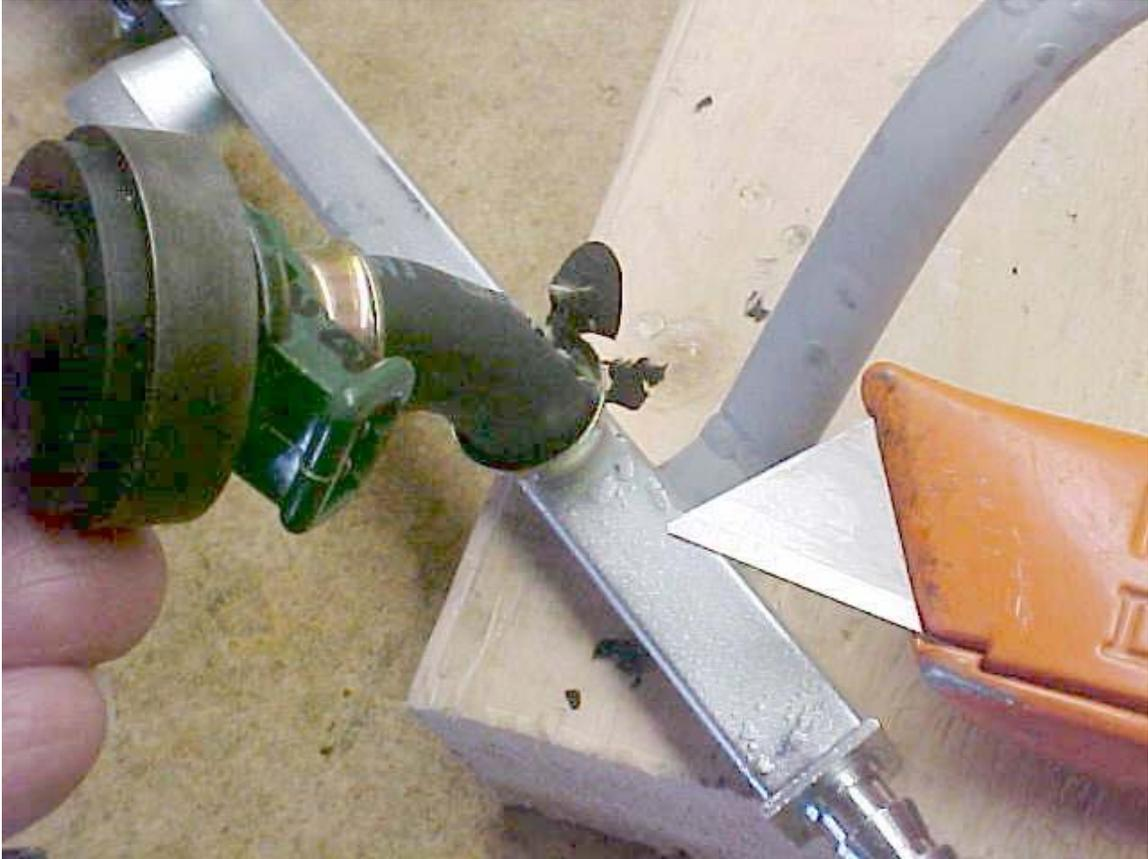
**Figure 11 Removing injector hose**
