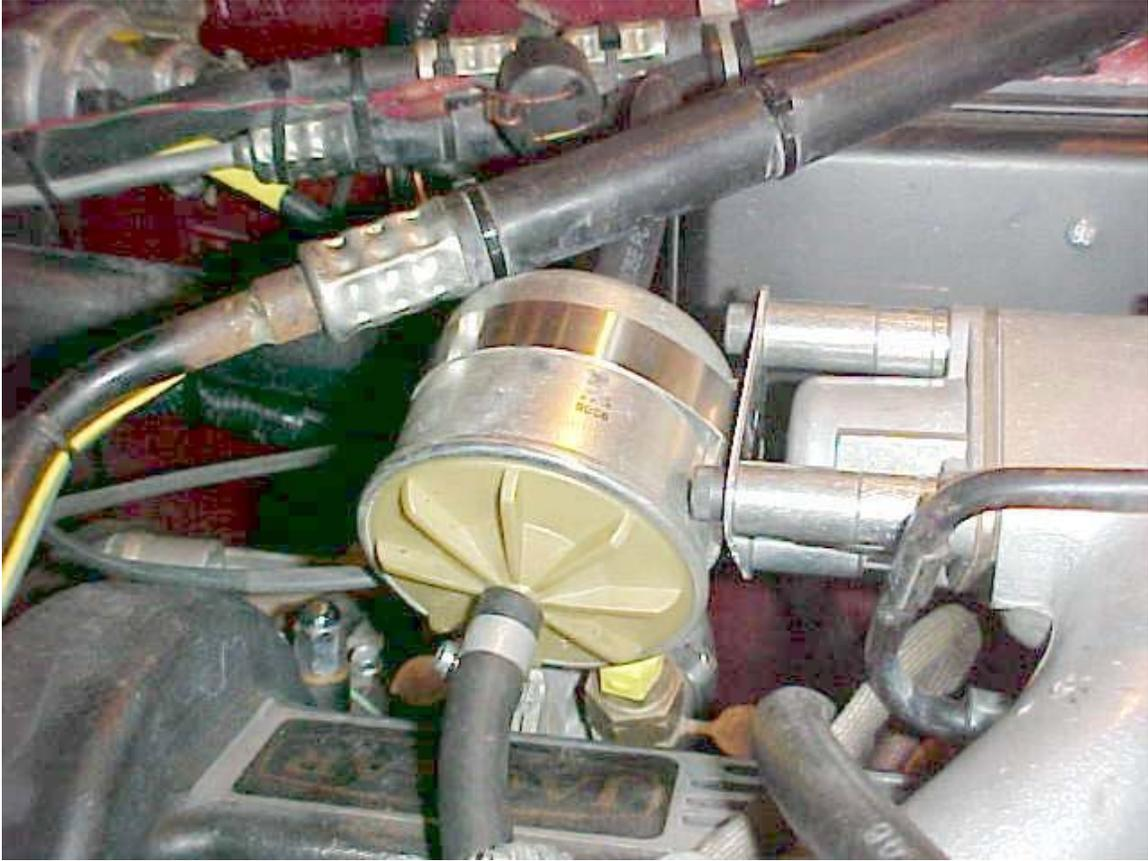
**Figure 6 Relocated fuel filter**
