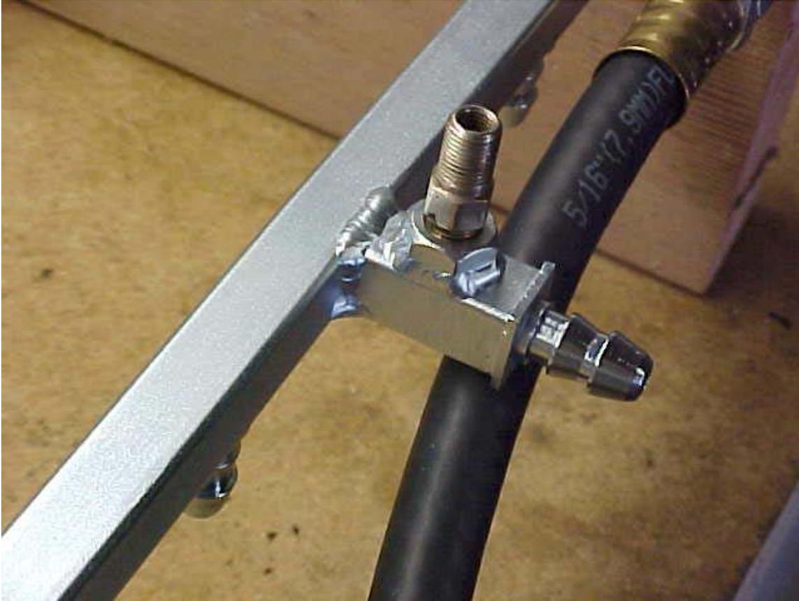
**Figure 3 Fuel pressure test port**
