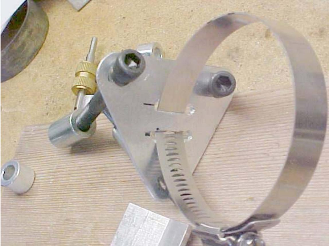
**Figure 7 Filter mounting bracket**
