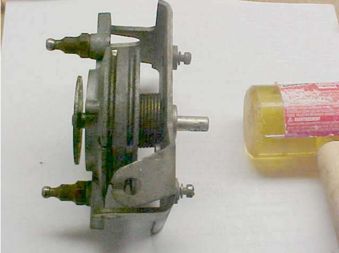
Figure 5 Removing the shaft
