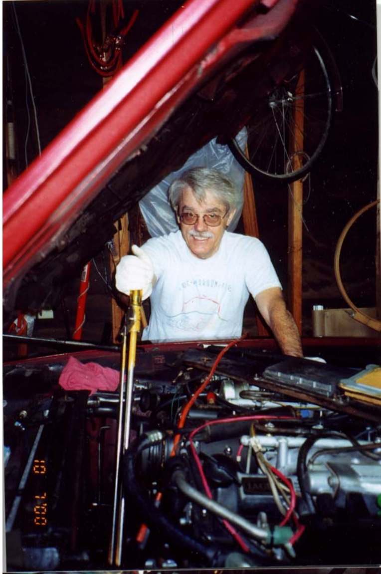
Figure 3. Tightening the damper bolt.
