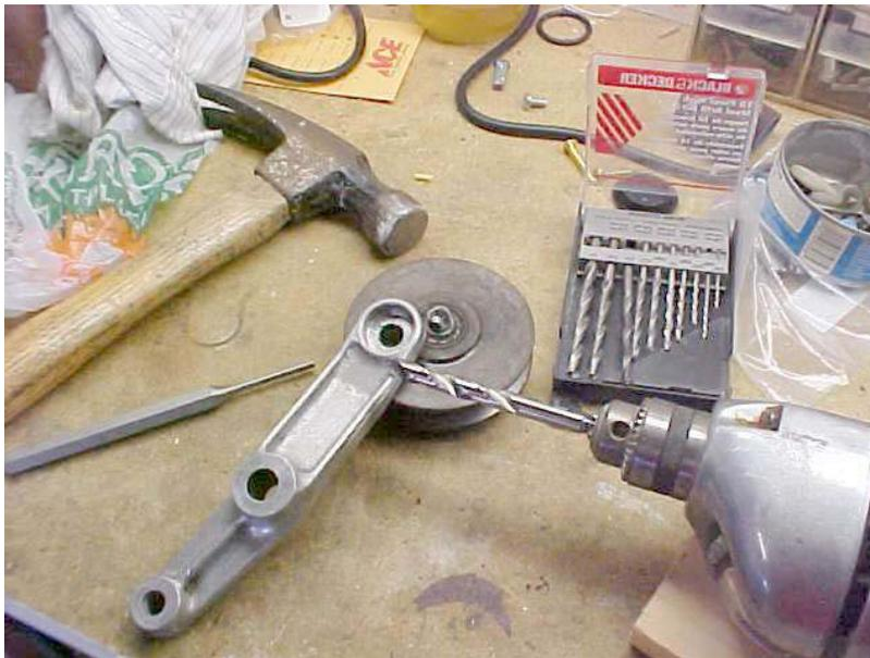
**Figure 4 Drilling the shaft out of the arm.**
