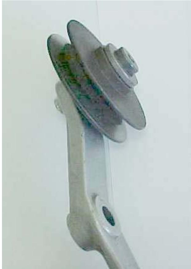
**Figure 8 Rebuilt Jockey Pulley on arm**
