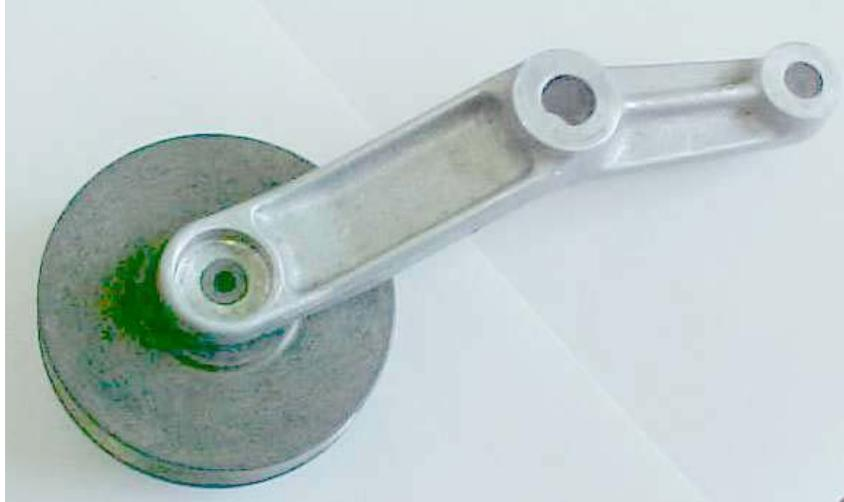
**Figure 1 Fan Jockey pulley and arm.**
