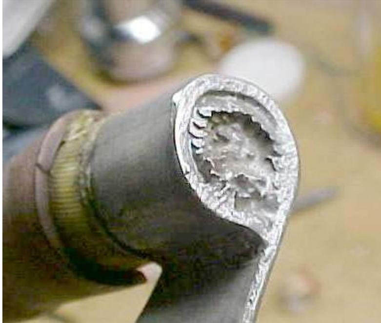
**Figure 5 Cable end after cleanup**
