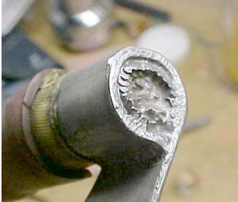
Figure 5 Cable end after cleanup
