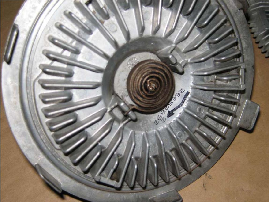
**Figure 3 Thermostatic element on HE clutch.**
