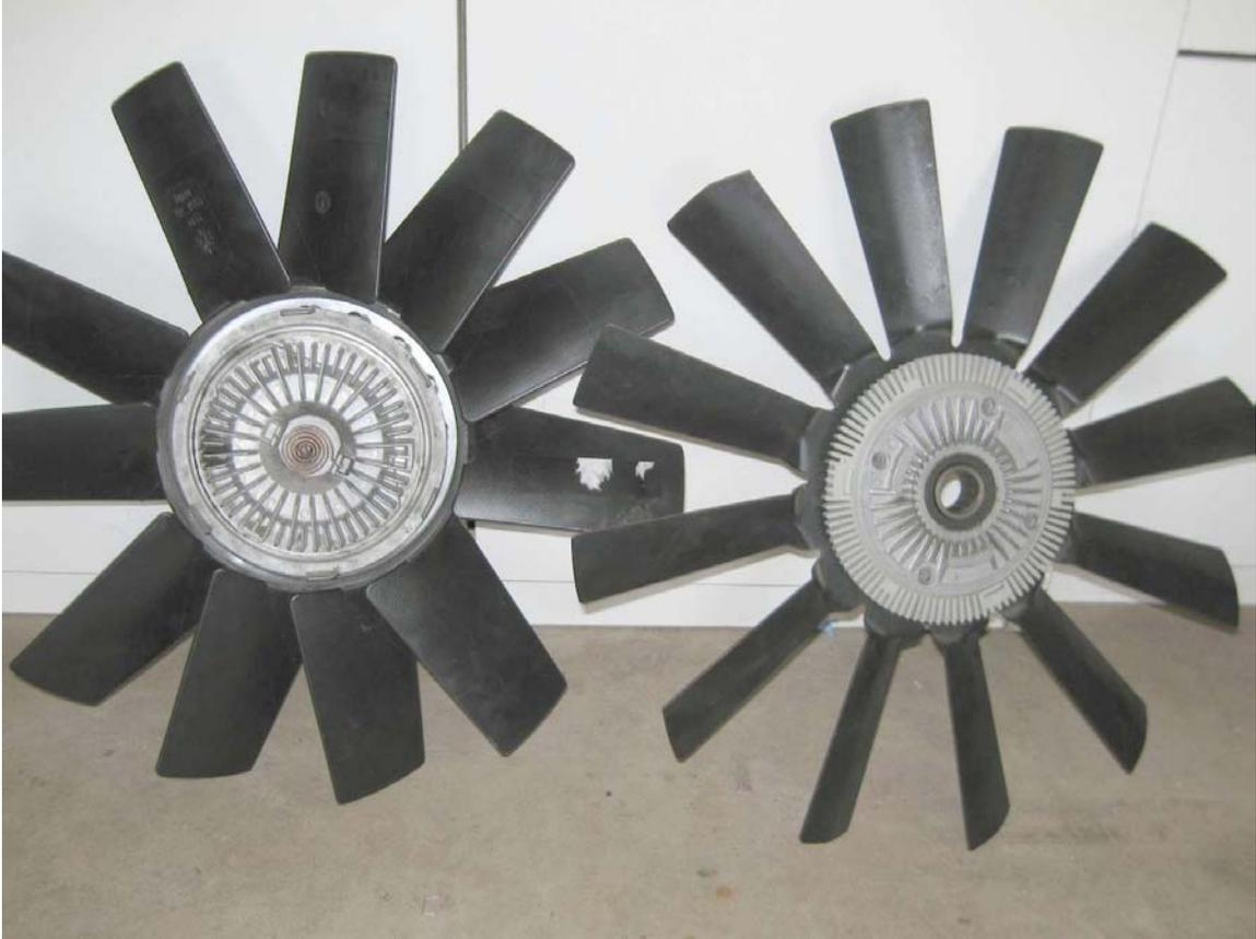
**Figure 1 HE (left) vs. preHE fans and clutches**
