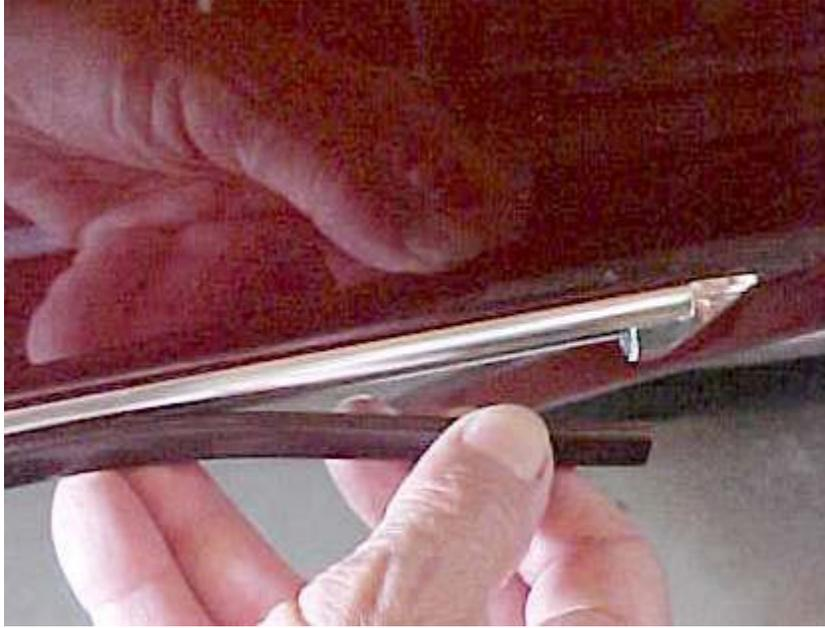
**Figure 1 Removing vinyl insert**
