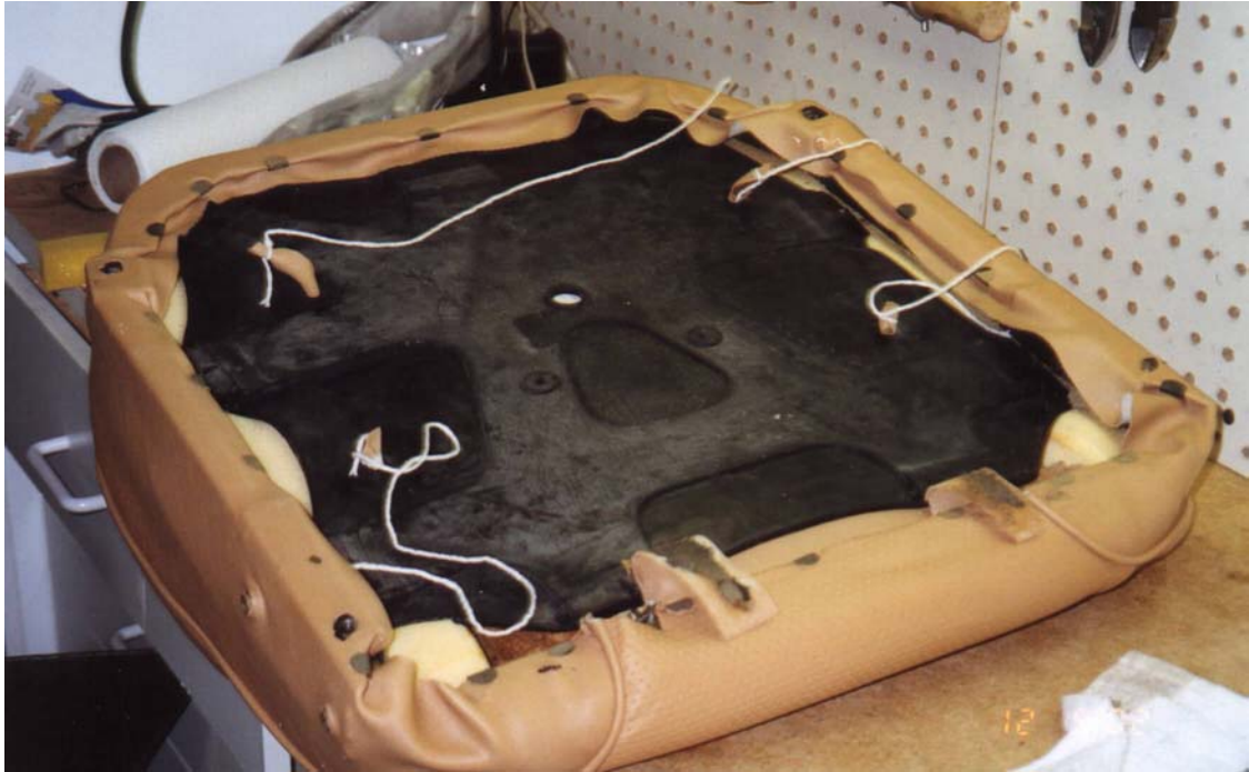
Figure 6 Installing the center pad.
