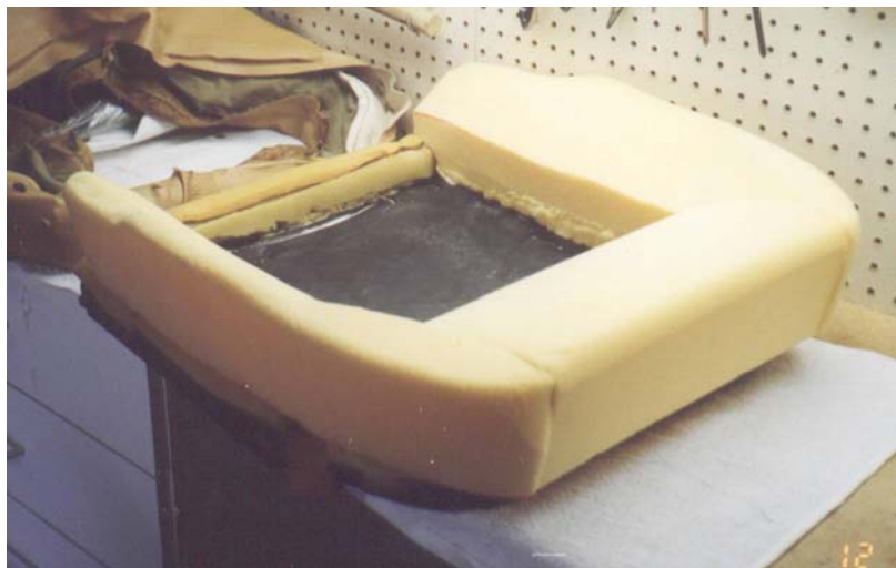
Figure 3 Bolster attached to frame.
